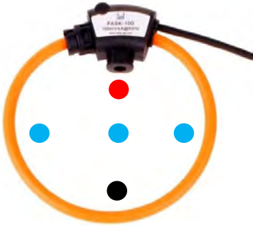
Figure 5: Position of primary conductor, with typical error values
