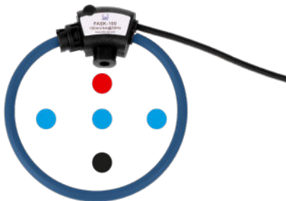
Figure 5: Position of primary conductor, with typical error values
