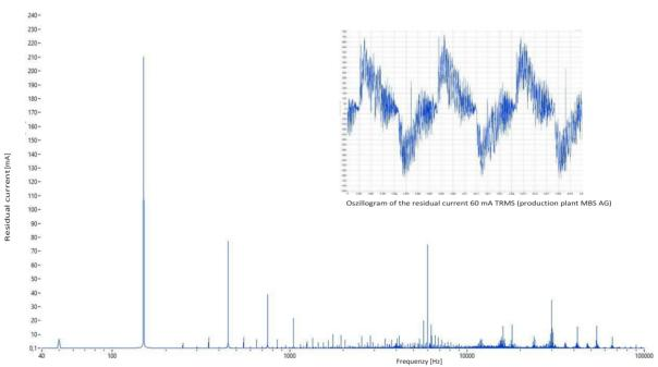
Frequency spectrum of the differential current at the production plant
