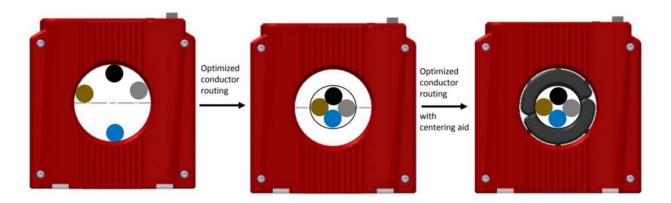
When the conductors are brought together with subsequent centering in the inner diameter, disturbances and inaccuracies can be significantly reduced. A centering aid can be ordered as an accessory in order to implement this optimized conductor routing in practice. This consists of EPP foam (expanded polypropylene) and is cut to theappropriate diameter with a sharp knife. If necessary, the individual conductors can also be brought together with cable ties before and after the passage.
