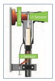
For first installation of new ring main units the current sensor on the upper left side is used, which is mounted over the bushing of the line.
