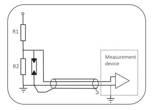
The voltage sensor based on the principle of an ohmic divider, which is adjusted in the factory to the guaranteed accuracy level. It is only necessary to know the ohmic part of the input impedance of the measurement device, due to the sensor is insensitive against changes in the capacitance.
