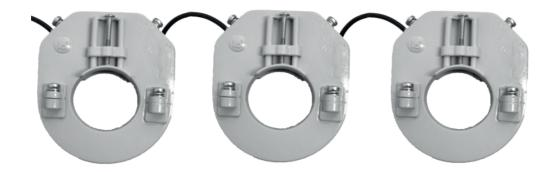
The earth fault sensor consists of 3 divisible sensors. The signal is delivered from the main sensor in the middle. Complimentary sensors on right/left deliver the signal for calculation of residual current.
