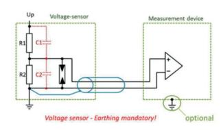
Due to electromagnetic compatibility, it is mandatory to adept the connection configuration to the measurement device.
