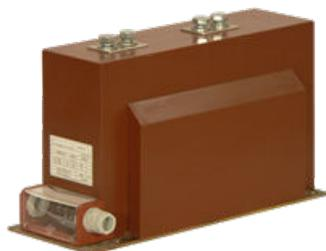
Medium-voltage current transformers for indoor application, which are converting multiple primary currents proportional and in-phase into measurable and standardized secondary currents.
