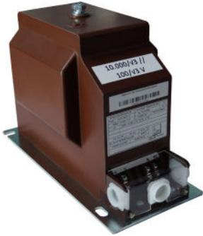
Medium-voltage voltage transformers for indoor application, which are converting one or more primary voltages proportional and in-phase into measurable and standardized secondary voltages. These transformers are fully resin-hardened in polyurethane.
