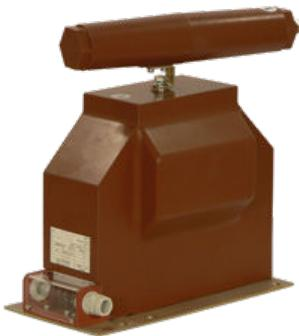
Medium-voltage voltage transformers for indoor application, which are converting one or more primary voltages proportional and in-phase into measurable and standardized secondary voltages. These transformers are fully resin-hardened in polyurethane.
