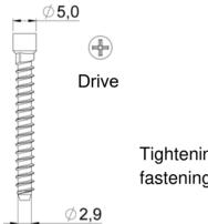
Tightening torque of fastening screw: 0.5 Nm
