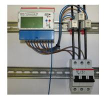
The combination of three single-conductor current transformers to a three-phase current transformer set, centre spacing 17,5 mm. CTs for phase L1 and L3 are mounted on top hat rail by means of snap-on mounting (order nr. 55018), the CT for phase L2 can be clipped on the other two CTs.
