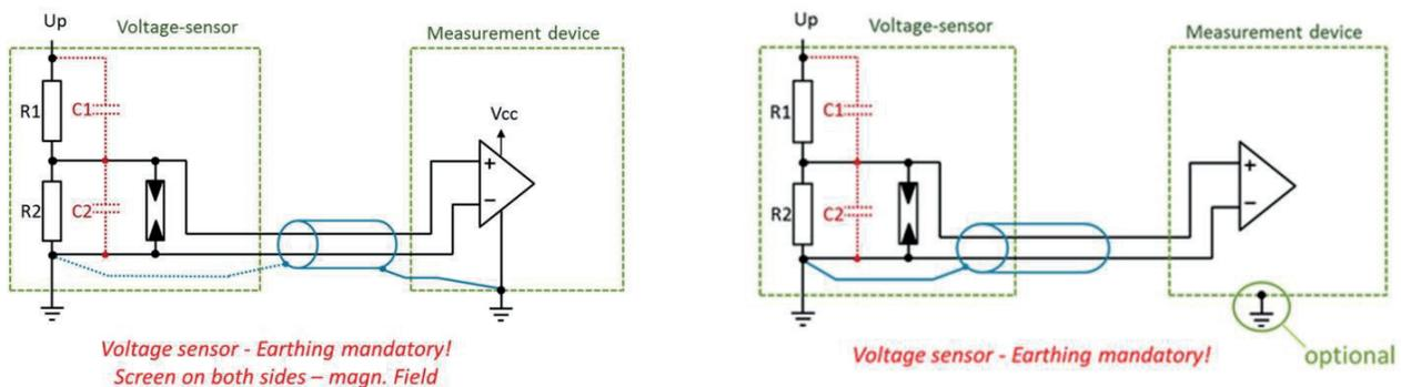
Due to electromagnetic compatibility, it is mandatory to adopt the connection configuration to the measurement device.
