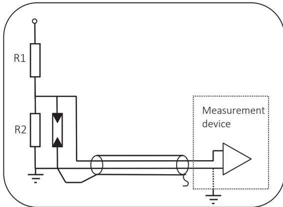
The voltage sensor based on the principle of an ohmic divider, which is adjusted in the factory to the guaranteed accuracy level. It is only necessary to know the ohmic part of the input impedance of the measurement device, due to the sensor is insensitive against changes in the capacitance.
