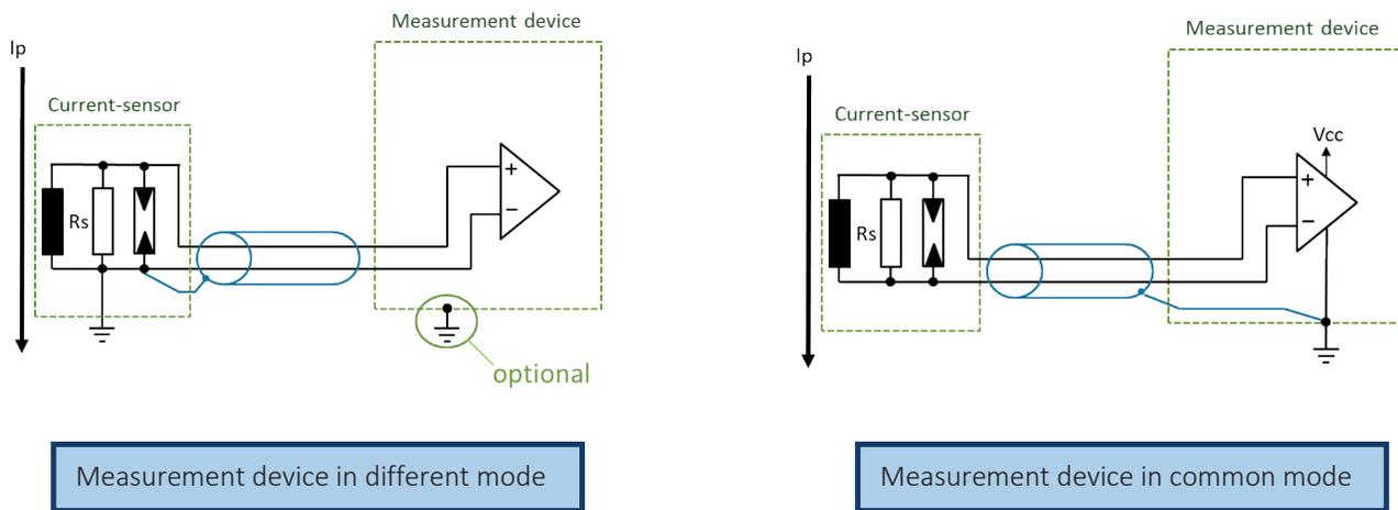
Due to electromagnetic compatibility, it is mandatory to adapt the connection configuration to the measurement device. The current sensors could be applied on measurement devices, doesn't matter which mode is used common or differential mode.
