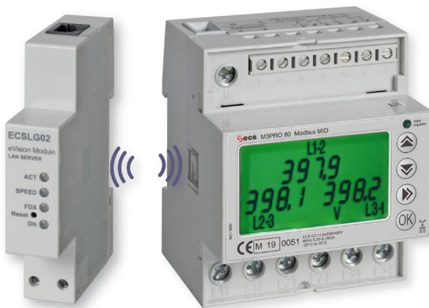
The universal modules of communication are used to enhance the Meters with additional communication functions. The units are installed directly next to the Meter and communicate via the infrared interface equipped on the side. Supported protocols are Modbus RTU, KNX, LAN-TCP/IP and M-Bus. The communication module receives data through an infra-red interface (IrDA) - placed on its side at 9.600 baud which is coupled with the mirror interface placed on the measuring device.
