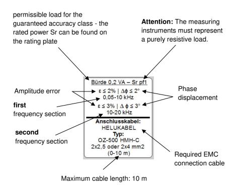
**Attention:** The instrument security factor FS only applies to the nominal load Sr on the main rating plate under 5.3.
